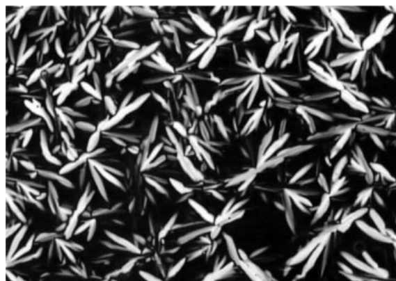
Figure 3. Optical texture of hexagonal columnar phase formed by the Schiff-base ligand \text{LH}_3 at 58 °C.
